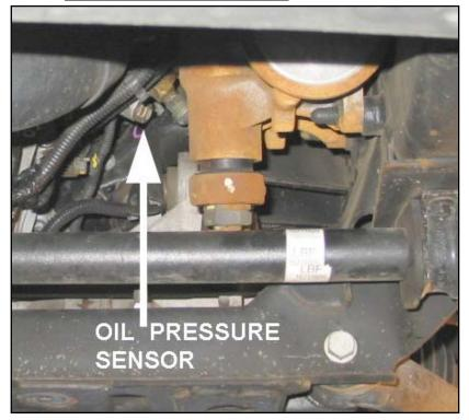
Remove the front skid plate from the bottom of engine and locate the oil pressure-sending unit on left side of engine block by the steering box.
