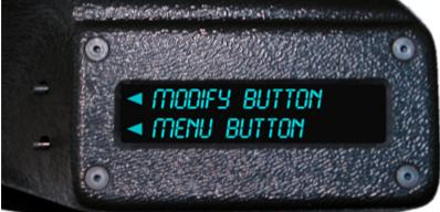
To change the settings and set alarm values there are 2 buttons on the side of the display, the bottom (MENU) button cycles through the different modes and the upper (MODIFY) button controls the setting of the values.
