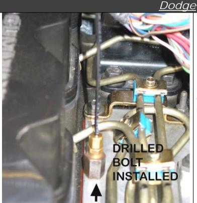
Locate and remove one of the intake plenum-to-manifold bolts and install the supplied boost fitting assembly with this kit and tighten to proper specifications. (These bolt holes all open into the intake manifold).
