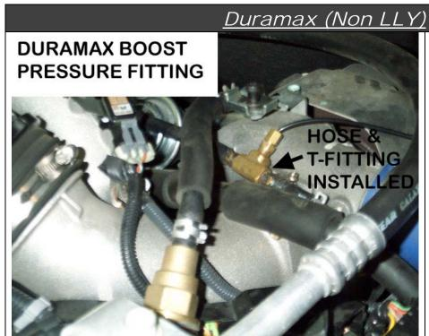
Locate the turbo wastegate hose and follow it along to the plenum.
