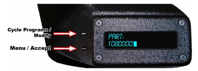
This X Monitor comes with alarm, peak memory, memory clearing and brightness functions that can be accessed and set by the two buttons on the side of the display.
