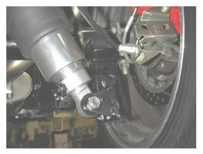
7. Bolt the lower axle bracket to the leaf spring pad using the 9/16" U-bolts and hardware supplied. Bolt the lower Shockwave mount to the axle bracket using the 5/8" x 1 1/4" bolts and Nylok nut.
