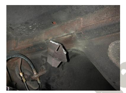
3. One more thing needs to be removed before starting the assembly; it's the pinion snubber and mount. For a clean cut use a cut off wheel and smooth any burrs.
