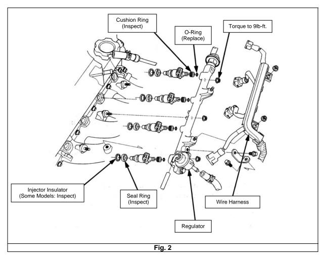
j) Inspect all seals, o-rings, and washers. If any of these components look at all worn or damaged, then replace with genuine Honda parts.
