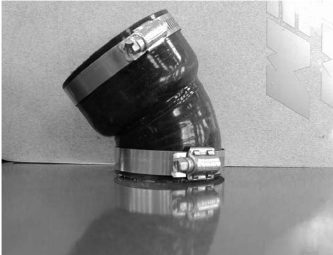
a) Assemble the 45 degree coupler as shown with hose clamps attached loosely.
