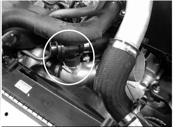
f) Insert BOV outlet into the BOV hose. Make sure you rotate the BOV toward the firewall, so that it clears the coolant hose.
