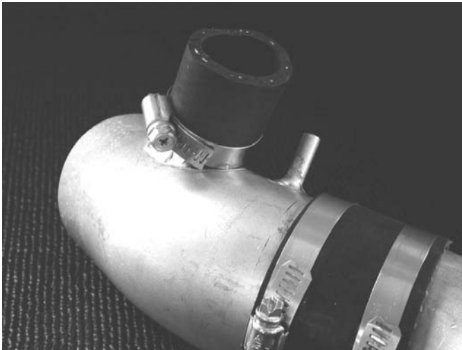
e) Trim hose to 1.5" Attach Blow Off Valve (BOV) hose to inlet pipe and rotate as necessary for proper fit. Secure with hose clamp.
