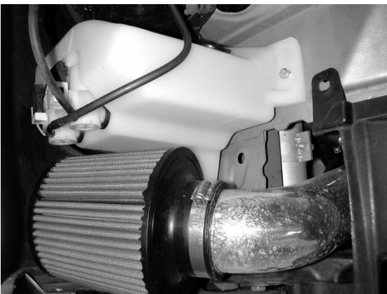
K) Install the AEM air filter onto the lower end of the inlet pipe.
