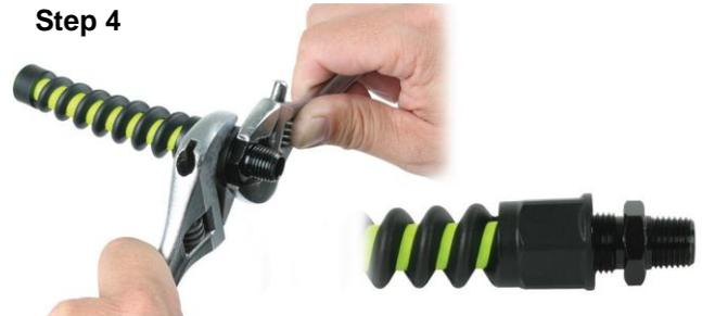
Place a wrench on the bend restrictor hex. Place another wrench on the male fitting. While keeping the male fitting stationary, tighten the bend restrictor until snug.
