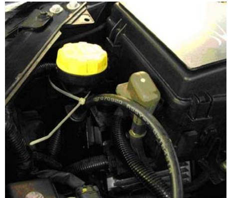
Step 3. Insert 4 push fasteners to secure the radiator cover. If the lip of the cover appears high in the front in the area near the blue cap, be sure the cover is not hooked under one of the protrusions on the windshield washer fill tube. Adjust if necessary.
