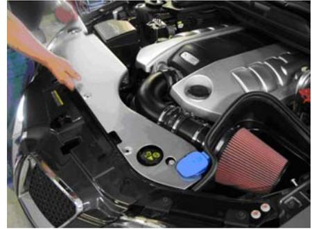
Step 2. If necessary, Align the yellow coolant tank cap with the cut out in the radiator cover. Use supplied cable ties to align the coolant neck.
