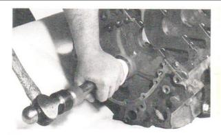
Place nylon cone in first bearing housing and drive bearing out. WARNING: Wear safety goggles. Loosen driver assembly to relieve pressure and pull tool back through he next bearing to be driven. Repeat above steps until all bearings are removed.
