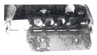
Operate tool from front of block. Insert into rear bearing and tighten until snug in bearing. (over)
