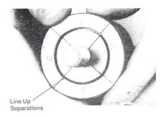
Check to insure that separation lines between segments of expanding driver line up with separation lines on the expander assembly as above.
