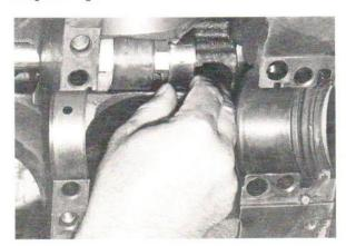
Reduce the expander assembly to its smallest size before installing bearings. Check the separation lines for proper alignment as in figure 2, page 1. Insert tool from the front of the block through the cam bearing housings until immediately in front of the rear bearing housing. Place bearing on expanding driver and tighten until bearing is held firmly. CHECK THE MANU-FACTURER'S SPECIFICATION TO MAKE SURE THE OIL HOLES IN THE BEARING ARE POSITIONED IN THE PROPER LOCATION.
