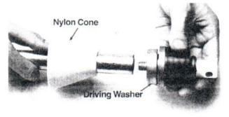
Place nylon cone over the driving bar. Then select the proper driving washer from the driver range table (see page 2). It is important to use the proper driver washer to prevent damage to the expander assembly. Place the driving washer over the threaded portion of the expander assembly. Screw expander assembly with driving washer into driving bar. (The driver bar extension may be needed for removal of the rear bearings.)
