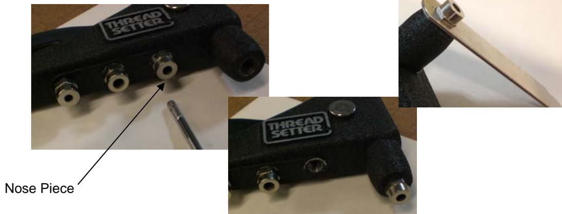
6. Thread Thumb Screw into rear of gun all the way. Then thread Rivet Nut onto end of Mandrel in the direction shown until it stops.
