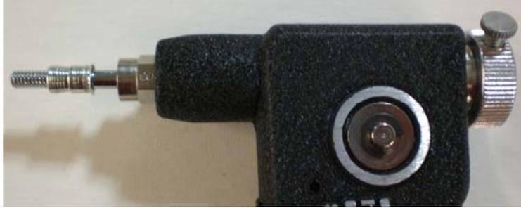
7. Back the Thumb Screw out until the Rivet Nut is flush with the Nose Piece. **Note:** Make sure the gun handle is in its released position.
