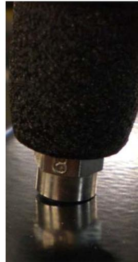
9. Unscrew the Mandrel from the Rivet Nut by loosening the Thumb Screw.
