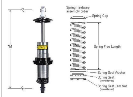
\*M = Proper measurement of shock length, extended, compressed, and shock ride height are taken from the centerline of the top shock mount to the centerline of the lower shock mount.
