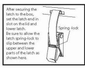
When the upper latch tab is in position and the spring-lock is protruding, simply push the lower latch end all the way down and the spring-lock will pop into place and secure the box. To open simply apply slight pressure upward on the spring-lock to release tension.
