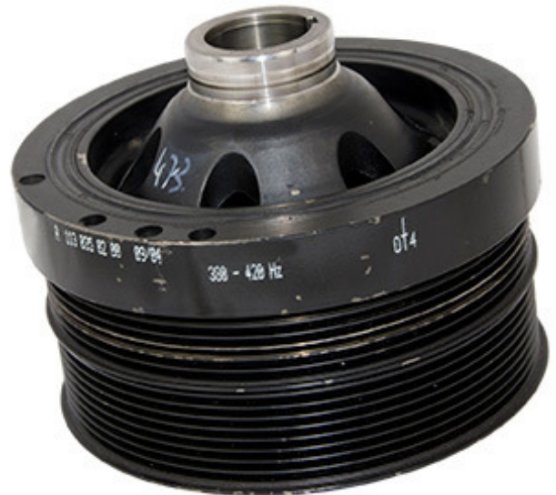
OEM harmonic balancer with frequency range stamp. It controls torsional vibration in a narrow range between 380 to 420 hertz.
