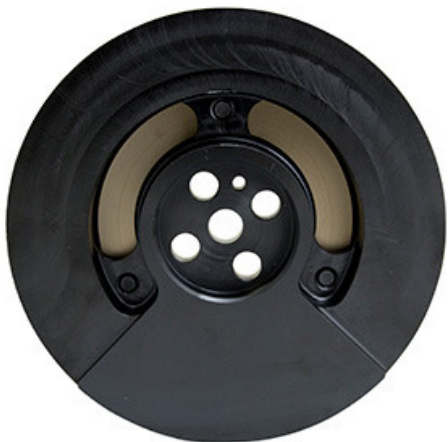
External balance. Note the large counterweight mass CNC machined into the housing. Fluidampr #800221 for 6.7L Ford Power Stroke applications.
