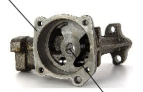
Full flow lubrication allows the driven shaft and gears to remain constantly lubricated while also providing a way for the aerated oil to escape.
